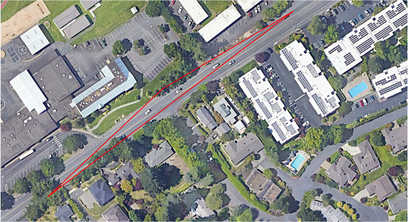
FIGURE 4. APPROXIMATE SIGHT TRIANGLE REQUIREMENT FOR EASTERN DRIVEWAY (350 FEET IN EACH DIRECTION)
